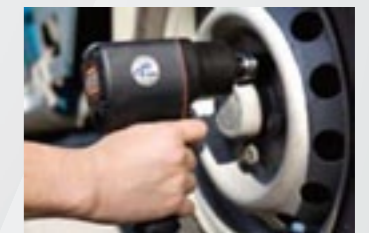
► Operation of 1/2" Impact Wrench with Torque Controlled
